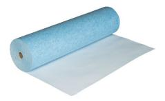
PrimaCover Active is a self-adhesive and breathable, polyester, non-woven covering. The multi-layer membrane on the upper side allows moisture to escape and prevents the ingress of liquids. It regulates moisture and has been specially developed for floors that are sensitive to moisture, such as natural stone and cast floors.
